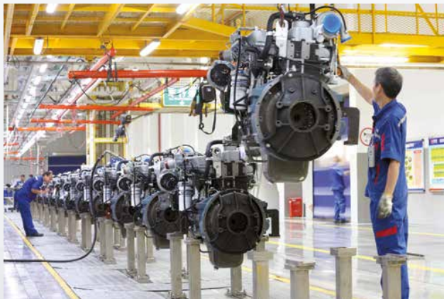
Final inspection before Engine off-line.
