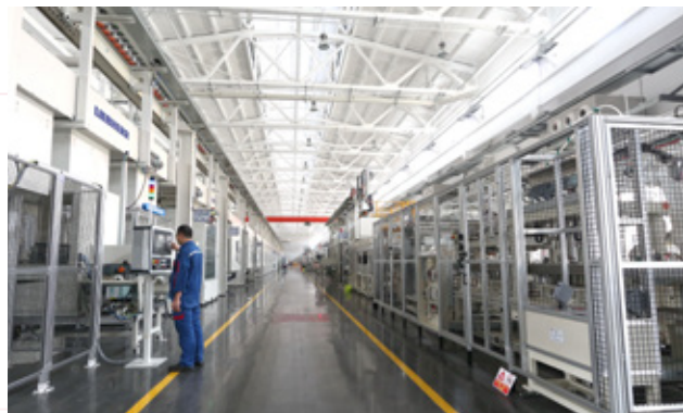
Finish Machining Line for National VI compliant Engine YCK05/YCK08 cylinder head machining.
