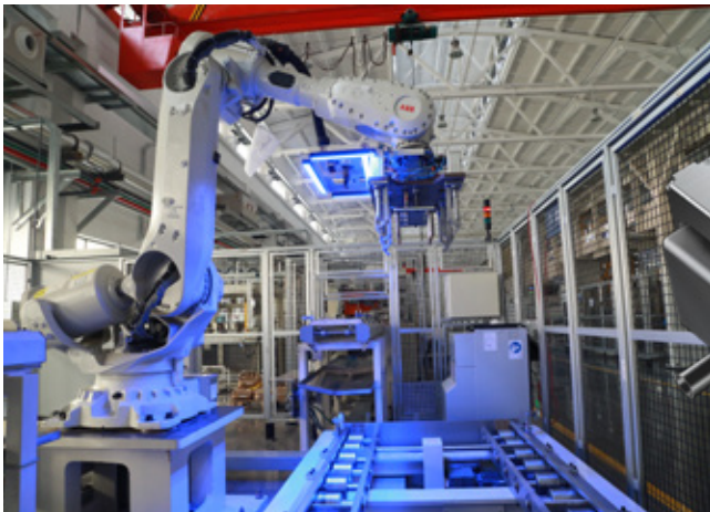
Yuchai National VI Engine Machining Line - robot station at material feeding with QR-code scanning.
