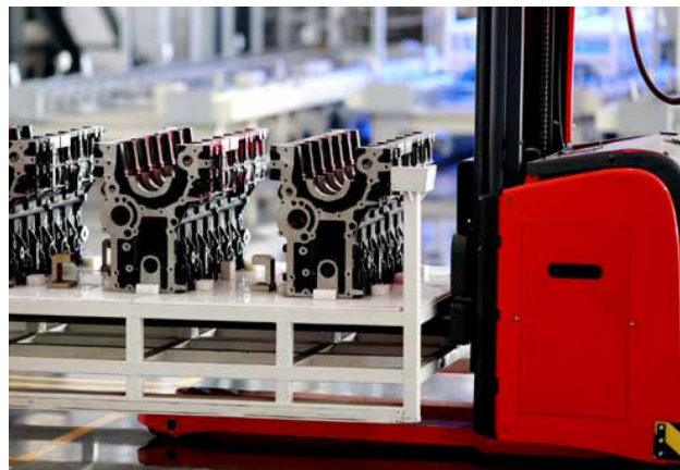
AGV are widely used for logistics support, such as sending engine components to the lines, or collection after machining.
